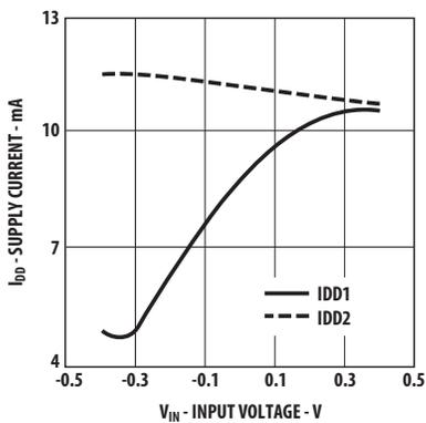
Figure 12: Input Current vs. Input Voltage
