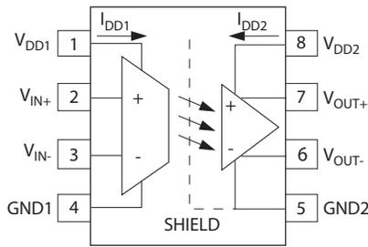
**NOTE:** A 0.1- $\mu$ F bypass capacitor must be connected between pins 1 and 4 and between pins 5 and 8.
