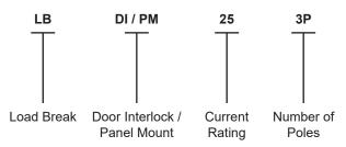
Door Interlock / Panel Mount : DI = Door Interlock and
