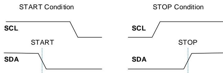
Figure 5. START and STOP Condition Waveform
