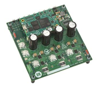
motor driver. As part of the motor development kit, the power board is compatible with the power Universal controller board enabling high-end control strategies and Al capabilities for industrial motor control. The complete kit is Strata enabled and the graphical user interface can be used to set control parameters for the motor drive.
