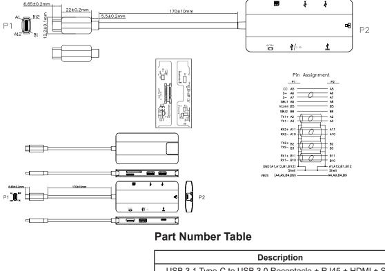
Part Number USB 3.1 Type-C to USB 3.0 Receptacle + RJ45 + HDMI + SD/ Micro SD + USB Type-C Receptacle Data or PD Charging Adapter
