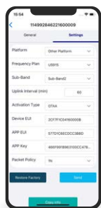
3 Join LoRaWAN network
