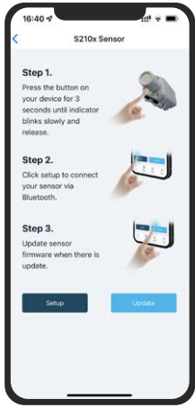
Configure sensor and do OTA
