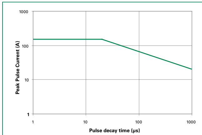
Figure 1: Non-repetitive Peak Pulse Current vs. Pulse Time
