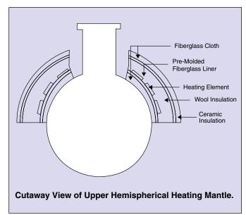
**UPPER HEMISPHERICAL MANTLES** are ideal for preventing vapor condensation in the upper half of the flask. The opening holds 1-, 2-, or 3-neck flasks.
