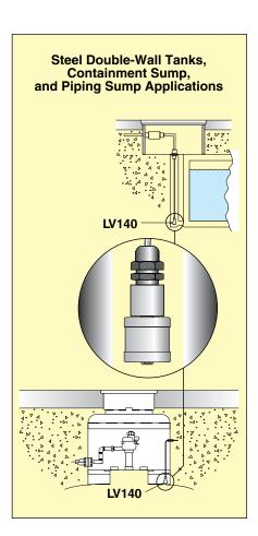
**Note:** The LV140 sensor is a non-voltage-producing device and does not contain energy-storing components. However, since primary use is in hazardous locations, an appropriate intrinsically safe (IS) interface device is required for its use.
