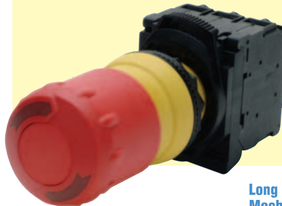
OMPBD7P-MT34PX01, plastic pushbutton, 30 mm mushroom, red, maintained operation with 1 NC contact.
