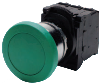
OMPBD7M-MM43PX01, metal pushbutton, 40 mm mushroom, green, momentary operation with one NC contact.
