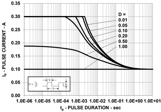
Figure 9: Pulse handling capability at  $T_s = 100^\circ\text{C}$ . (820nm, 830nm, 870nm)
