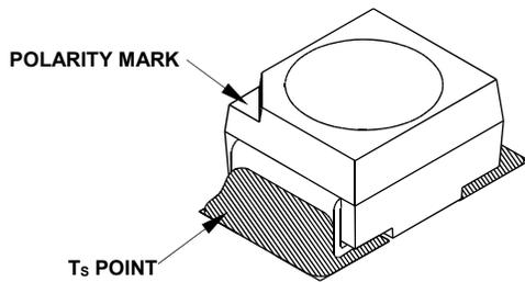
$T_s$  can be easily measured by mounting a thermocouple on the soldering joint as shown in preceding figure, while  $R_{\theta J-S}$  is provided in the data sheet. Verify the  $T_s$  of the LED in the final product to ensure that the LEDs are operating within all maximum ratings stated in the data sheet.
