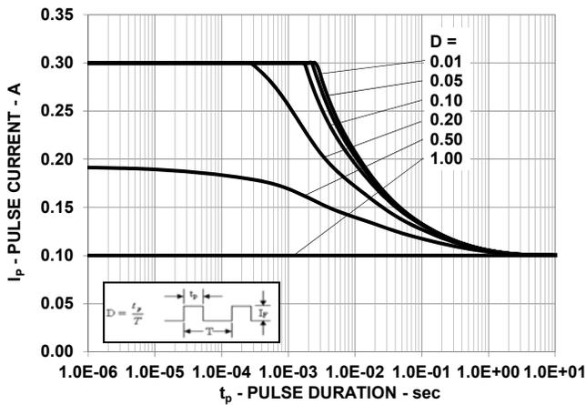
Figure 11: Pulse handling capability at  $T_s = 100^\circ\text{C}$ . (890nm)
