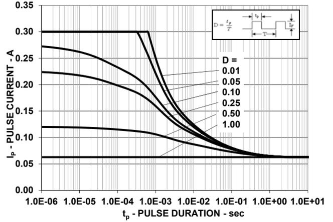
Figure 10: Pulse handling capability at  $T_s < 94^\circ\text{C}$ . (890nm)
