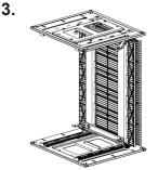
Take the movable side board (3) into the rack in accordance with upper and lower movable groove. Notice: the four gear seat must close to gear rack, then pull back to elongated slot of the bottom board. (Picture above)
