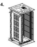
Pull movable side board to the end of moveable groove (picture above)
