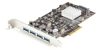
This PCIe USB 3.2 Gen 2 controller card installs into an available PCI-Express x4 slot in your computer and enables you to upgrade your current system by adding four SuperSpeed USB-A (10Gbps) ports. The card features dual ASM3142 controllers with up to 20 Gbps of total bandwidth shared across all 4 ports.
