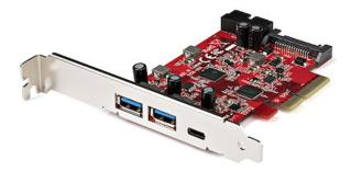
This 5-port USB 3.2 Gen 2x1 (10Gbps) combo card makes it easy to add to the performance and connectivity of your computer. The USB 3.2 card offers a USB Type-C port (10Gbps), two traditional USB Type-A ports (10Gbps), and a motherboard header (USB 5Gbps).
