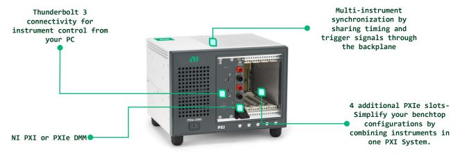
With the PXI DMMs, perform hand-probed, switched, and further automated DMM measurements with high accuracy and resolution. The PXI DMMs deliver fast, accurate AC/DC voltage, AC/DC current, 2- or 4- wire resistance, and frequency/period measurements, as well as diode tests. These bundles feature DMMs with up to 7.5 digits of resolution, 1000 V DC voltage range, 3 A current range and 1.8 MS/s sample rate.
