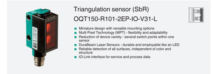
Switching diffuse mode sensor with measurement core technology, 150 mm detection range, red laser light, laser class 1, IO-Link, 2 x push-pull output, M8 plug
