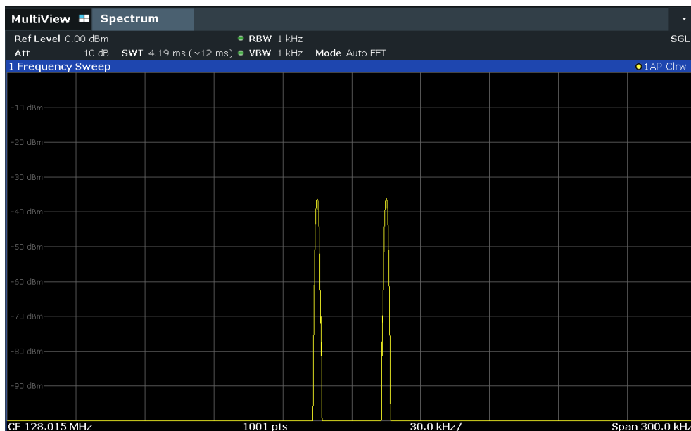
Figure 6-8: Measurement of two equally-leveled RF sinusoidal signals with a resolution bandwidth (1 kHz) which is significantly smaller than their frequency spacing
