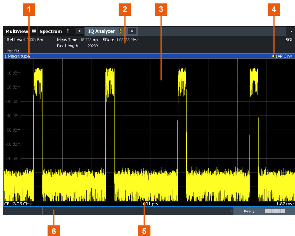
Figure 2-1: Screen elements in the I/Q Analyzer application
