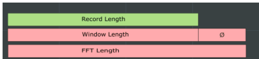
Figure 4-4: FFT parameters for single FFT calculation
