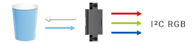
B5WC Color sensor using white LED as emitting light source and receives reflected light from the target object. Identify RGB ratio (Red / Green / Blue) and output the voltage by I2C communication.
