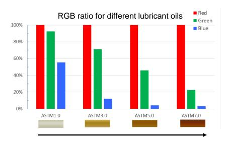
Lubricant oil color changes by degrading level
