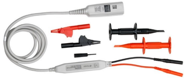
Figure 13. Keysight's N2818A 200-MHz differential active probe.
