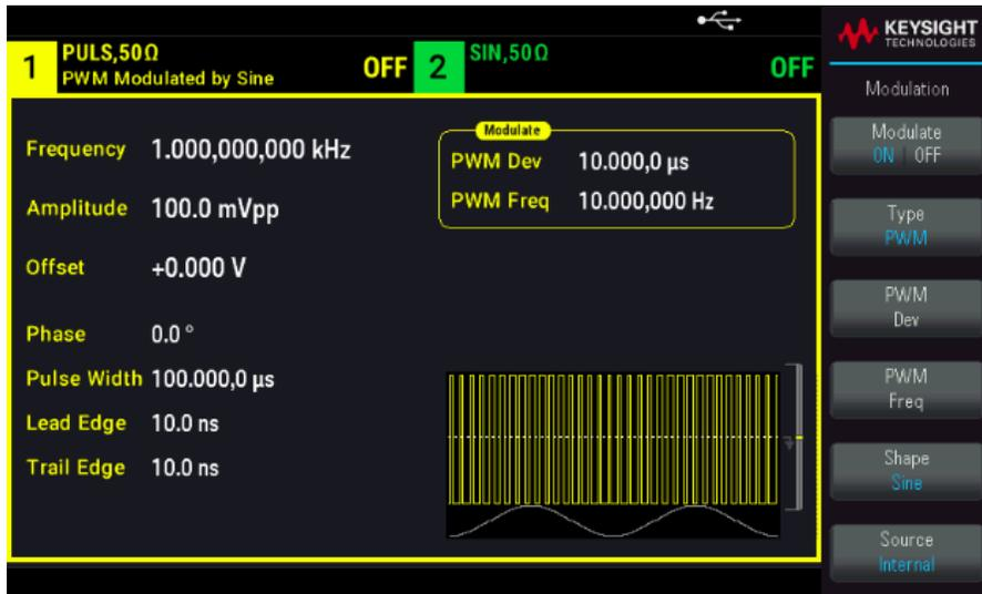
Figure 3. PWM modulated with standard sine wave
