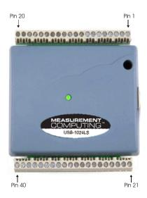
Figure 3-2. USB-1024LS screw terminal pin numbers
