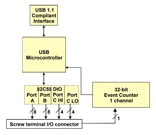
Figure 1-2. USB-1024LS functional block diagram
