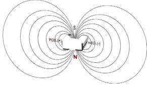
When a positive (+) voltage is placed on the terminal marked with the polarity dot and the opposite terminal is negative (-), the resulting current flow will create a magnetic south pole on the top side of the IHLP. Observing the polarity orientation when mounting the IHLP will insure the most consistent EMI reduction performance.
