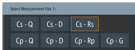
Figure 6-6: Example of selection editor for measurement parameter pairs
