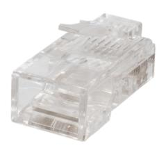
Category 5e Contractor Grade 5/FF/RJ45 Plug (PXSPDY5b): plugs are designed to simplify twisted pair terminations by allowing the wire pairs to be easily inserted through the plug and out of the front. This allows the installer to easily check the wiring order before crimping the connector. Twist is maintained more easily enabling a better performing crimp. Waste is minimised and the plugs are suitable for either stranded or solid wires.
