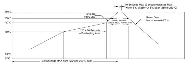
Following is typical SMD Pb-free reflow profile for soldering:
