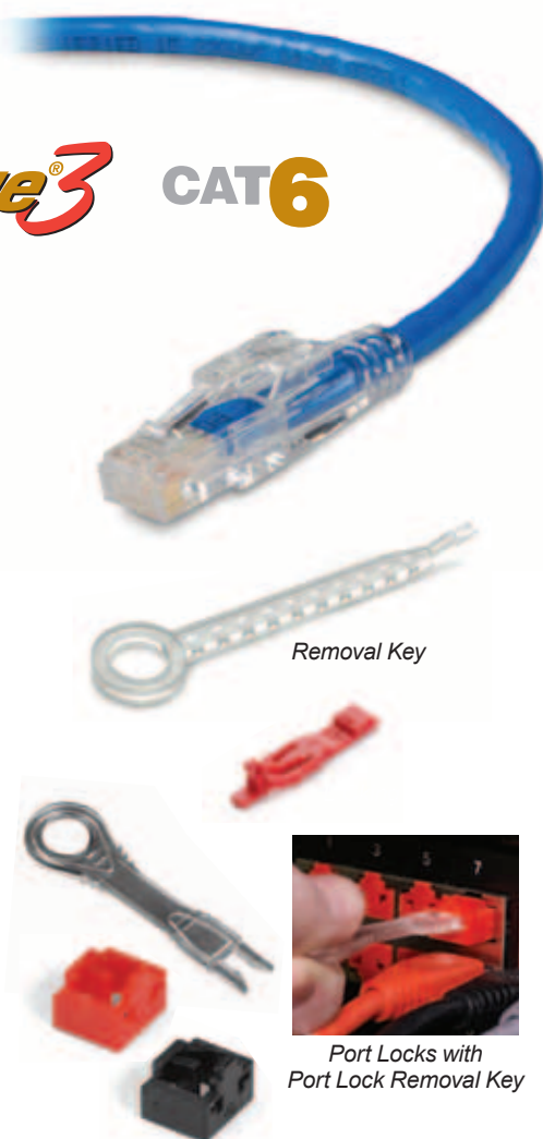
To unlock, insert the Key into the Pin until it clicks. Pull the Pin back and lift the Key to release.
