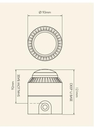
The Flashni is an audible and visual device which requires one single installation point. This greatly reduces installation and costs and is much less obtrusive than two separate devices. Versions are available with the sounder and beacon linked, or with separate terminals for independent operation.
