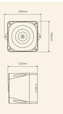
The Asserta Midi Sounder is versatile, compact unit that has been designed for industrial environments or areas where there is a requirement for a physically robust and well protected alarm is required. A range of supply options permit use with a wide range of fire and process systems.
