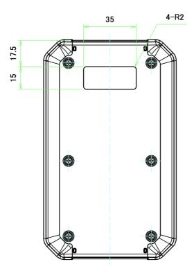
Maximum Carrier Board Dimensions (mm):
