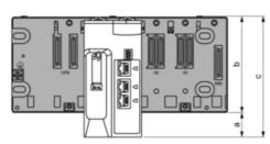
a: additional space below the rack to accommodate the height of the CPU. For an X Bus rack, the value is 30.9 mm (1.217 in.); for an Ethernet rack, the value is 29.49 mm (1.161 in.).
