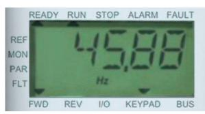
Backlit liquid crystal display (LCD)
