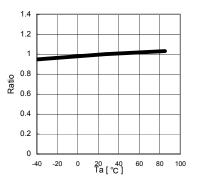
Fig.8 IOUT Temperature dependency (100 lx)
