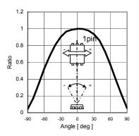
Fig.4 Directional Characteristics 1
