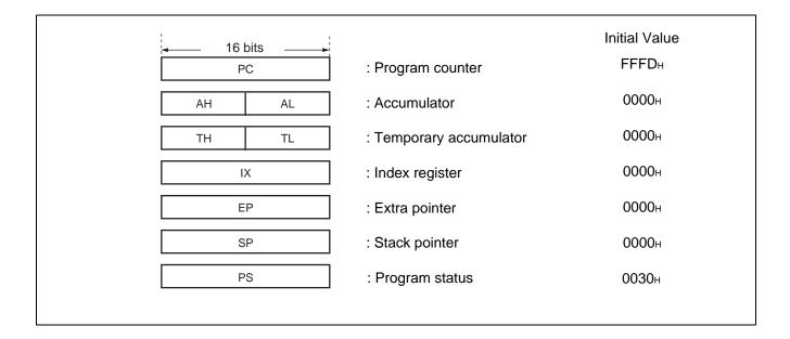
The PS can further be divided into higher 8 bits for use as a register bank pointer (RP) and a direct bank pointer (DP) and the lower 8 bits for use as a condition code register (CCR). (Refer to the diagram below.)
