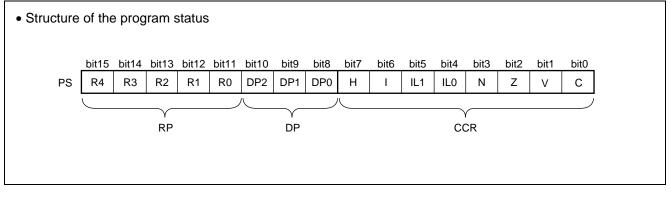
The RP indicates the address of the register bank currently being used. The relationship between the content of RP and the real address conforms to the conversion rule illustrated below:
