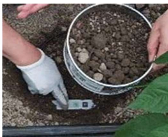
④ By fixing sensor, put more fine soil
