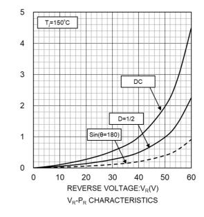
REVERSE POWER DISSIPATION:P<sub>R</sub>(W)
