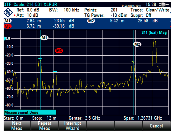
Wizard function support for common measurements: User-definable test sequences that reduce operating errors in the field
