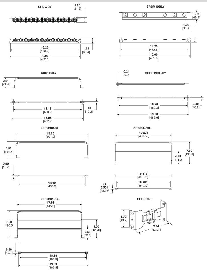
Dimensions are in inches. [Dimensions in brackets are metric].
