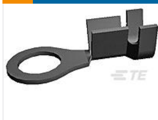
TE Part #40660 RING 164(4.17 MM) TERMINAL 18-14 AWG BR
