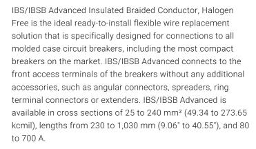
Manufactured in an ISO 9001 certified automated facility, IBS/IBSB Advanced is formed by weaving high-quality electrolytic copper wire to form a durable low voltage connector with maximum flexibility which allows for more compact power connections to circuit breakers. The IBS/IBSB Advanced allows users to reduce the total size and weight of the installation, improving both design flexibility and assembly aesthetics.
