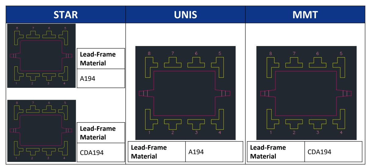
Note: C194, A194 or CDA194 Lead-Frame material are the same, it is just a MCHP internal labelling difference.
