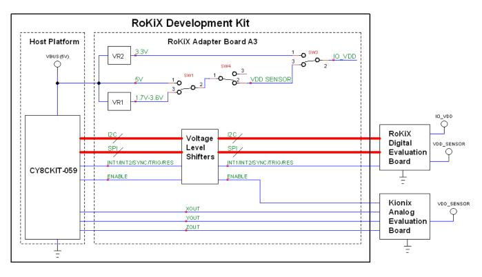
Figure 2. High Level Block Diagram of the RoKiX Development Kit
