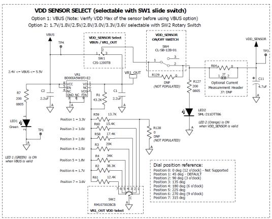
Figure 4. RoKiX Adapter Board A3 VDD Sensor Select
