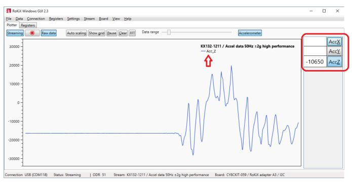
Figure 33. Plotter view with only AccZ sub-channel activated.
