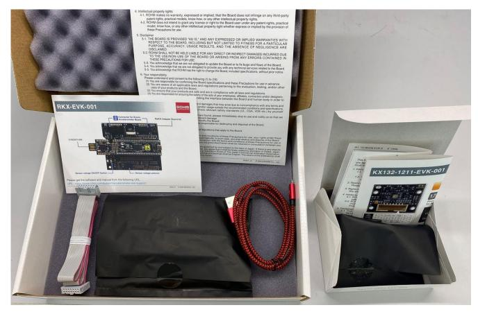
Figure 1. RKX-EVK-001 (Left) and RoKiX Digital Evaluation Board purchased separately (Right) shown here together
