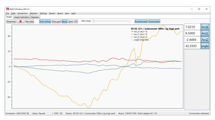
Figure 50. Plotter view with KX132-1211 inclinometer stream.
