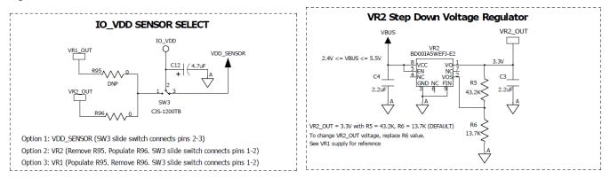
Figure 5. IO\_VDD Sensor Select and VR2 Voltage Regulator
