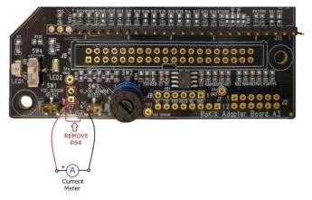
Figure 7. VDD\_SENSOR Current Measurement Recommended Connections
