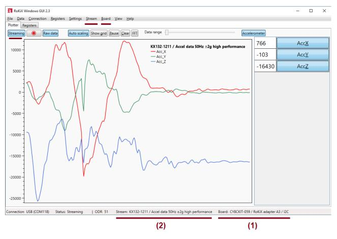
Figure 27. Plotter view with KX132-1211 motion displayed
