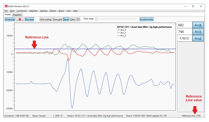
Figure 35. Plotter view with reference line enabled.
