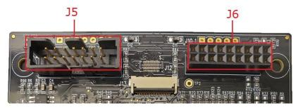
Figure 9. RoKiX Digital Evaluation Board Interface Headers
