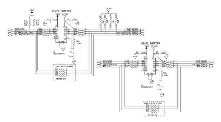
Figure 8. Voltage Level Shifters for I/O Signals
