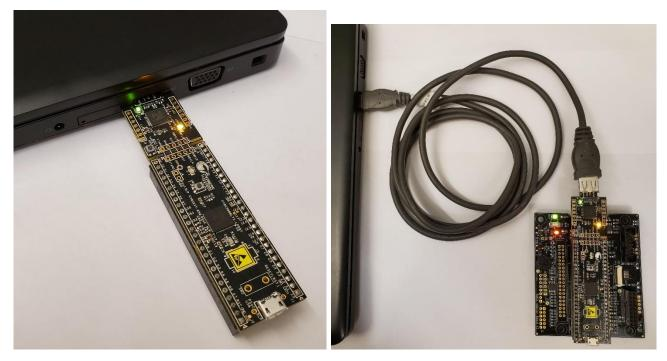
Figure 22. CY8CKIT-059 Prototyping Kit Connected to the PC
