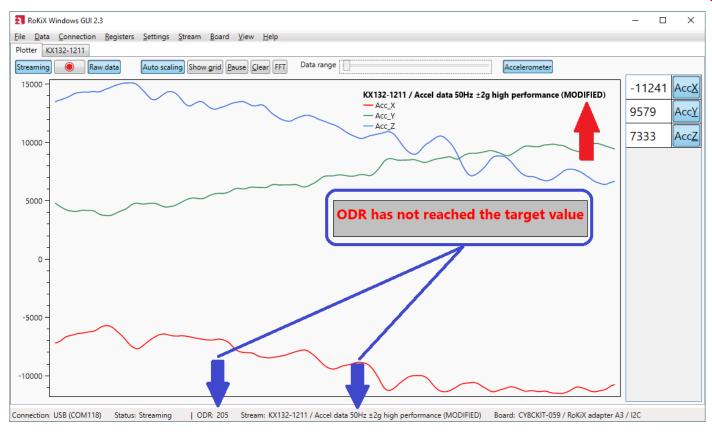
Figure 53. The Plotter View After Modifying the Register Values
