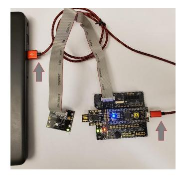
Figure 13. CY8CKIT-059 connected to PC (connection to the evaluation board is optional in this step)
