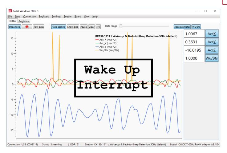
Figure 65. The plotter view with wake up triggered.
