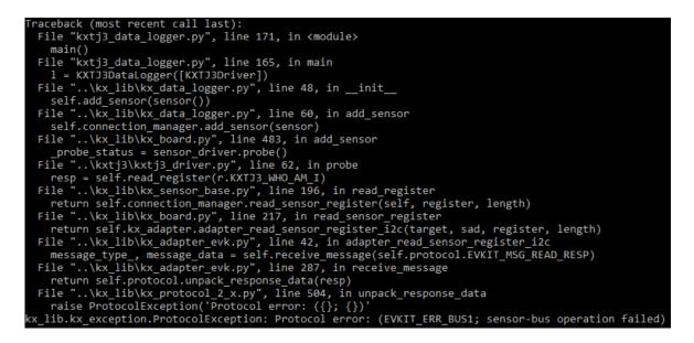
Figure 79. "EVKIT\_ERR\_BUS1; sensor-bus operation failed" error when running kxtj3\_data\_logger.py
