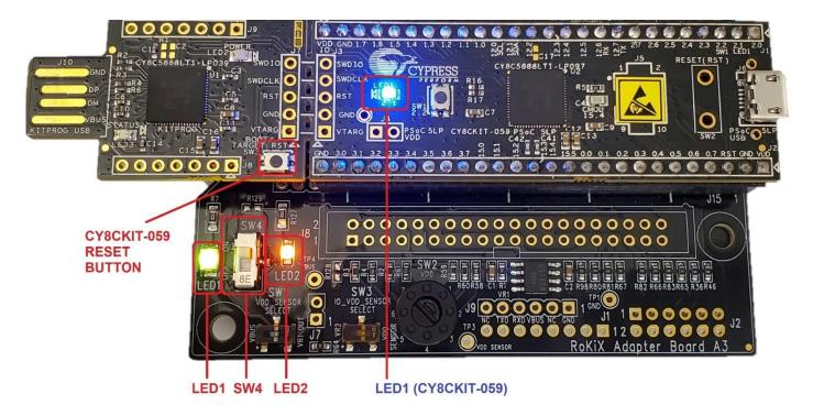
Figure 75. RoKiX Development Kit status: LED1, SW4, LED2, LED1 (CY8CKIT-059) must be ON
