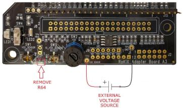
Figure 6. External Voltage Source Recommended Connection
