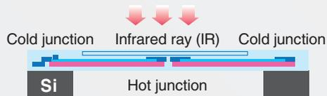
The sensor utilizes the seebeck effect in which thermoelectric force is generated due to the temperature difference that occurs across the junction points of two different types of metal.
