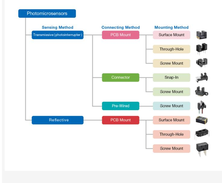
Typical applications of Photomicrosensors (photointerrupters)
