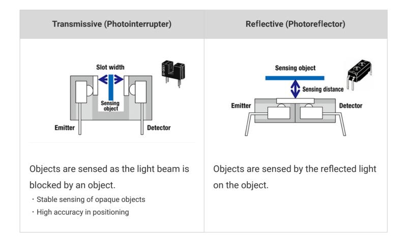
nsmissive(slot) Photomicrosensor(photointerrupter) detects objects by passing the et object through the emitted light beam from the aperture. This is ideal for applications of small object detection or accurate position sensing. A reflective Photomicrosensor detects the presence and absence of objects but also detects marked objects. This type is effective for realizing a low-profile design of a device or piece of equipment.
