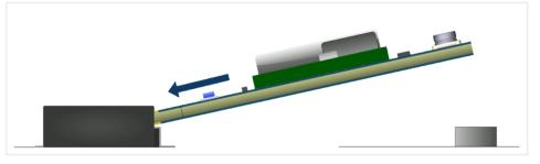
3. Apply some light downward pressure until the PAN9028 M.2 device is parallel to the host board and makes contact to the threaded insert.
