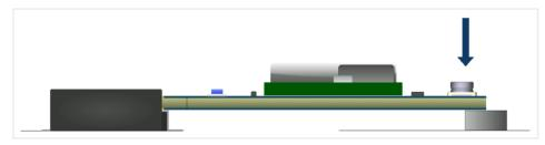
4. Insert a M2.5 x 4 machine screw into the mounting screw indentation (2) and the threaded insert.
