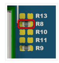
2. Place a 0 Ohm resistor (0402) for **R13** or bridge it with a solder blob.
