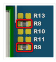
2. Place a 0 Ohm resistor (0402) for **R13** and or bridge it with a solder blob.
