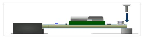
$\rightarrow$  The PAN9028 M.2 device is secured in place.
