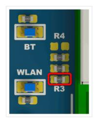
2. Place a 0 Ohm resistor (0402) for **R4** or bridge it with a solder blob.
