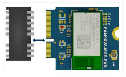
2. Insert the PAN9028 M.2 device into the socket slightly angled.
