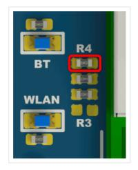
2. Place a 0 Ohm resistor (0402) for **R3** or bridge it with a solder blob.
