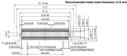
Note  $\boxed{1}$  Cross-hatched portions, totaling n places, indicate the ground circuits.
