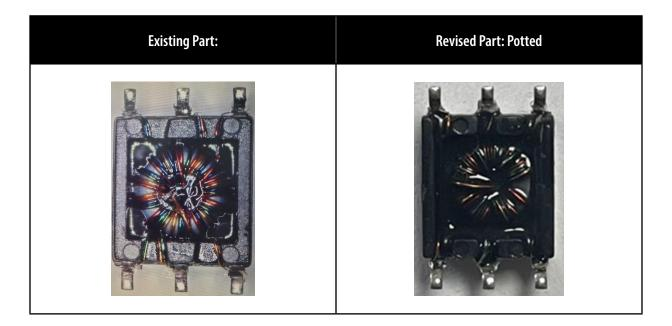
The form of the transformer will be changed due to the change to the case and potting described above. The fit and function of the affected part numbers will remain the same. The quality and reliability of the affected part numbers should be improved. The production lead time of the transformers will remain the same. Traceability will be maintained through the lot code and date code marking.
