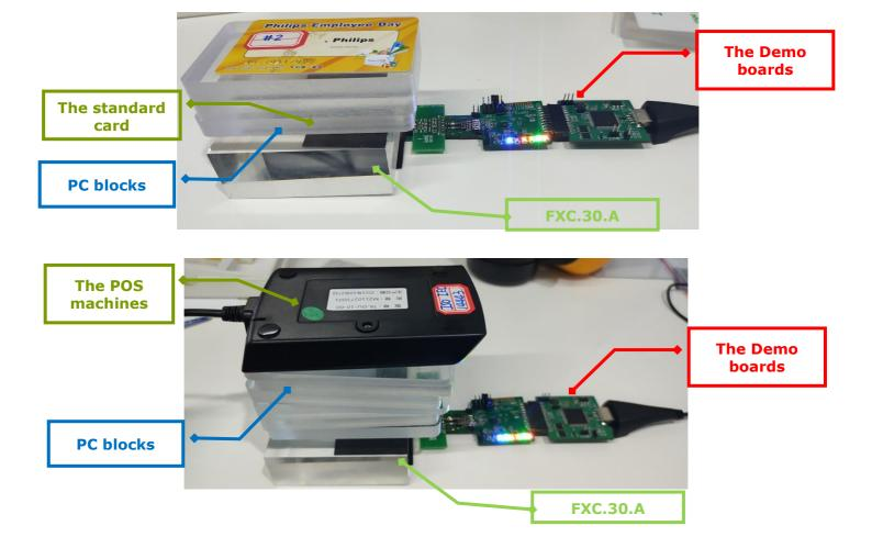
When the number of the PC material blocks are carefully adjusted until the reader can no longer read the sample, that's mean in this point the FXC.30.A cannot establish communication with the standard card or the POS machine, the thickness of the PC material block is the maximum interrogation distance of them.
