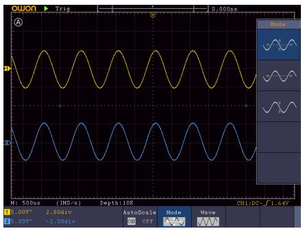
Figure 4-17 Autoscale Horizontal-Vertical multi-period waveforms
