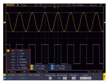
Figure 4-16 Time&Voltage Cursor Measurement
