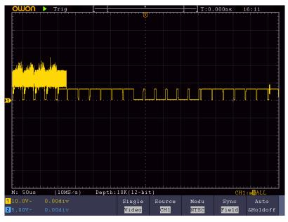
Figure 6-7 Waveform Captured from Video Field Trigger
