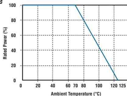
When the ambient temperature exceeds 70°C, reduce the rated power and current in accordance with the derating curve.
